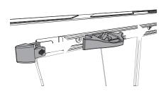
Reinstall any tie-down cleats and the end cap on both sides of the truck.
