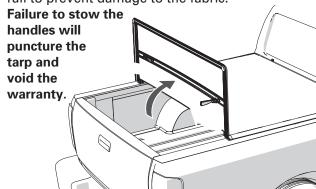
Fold the cover forward and fasten the straps to the front rail. Check that the straps are tight
