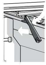
Rotate the clamp down and slide it to the truck bed rail.
