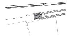
Insert the provided slide block into the cargo rail.
