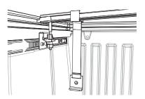
Move the slide block forward to the front bow of the cover.
